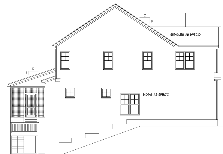
LEFT SIDE ELEVATION
