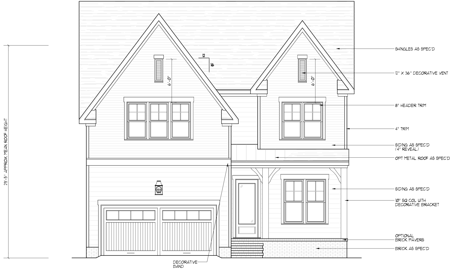
FRONT ELEVATION "A"
